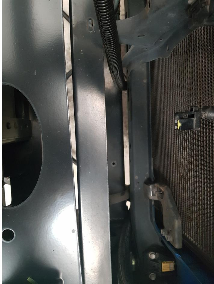
12. Lower the supplied cooler bracket into place and bolt (use factory bolt removed earlier) the cooler bracket to the vehicle using the (2) bolt holes on the bottom of the cooler bracket. See photo below for positioning of bracket and the location of the bolt on the left side. Loosely bolt the bracket to the vehicle using the left bottom bolt hole.
