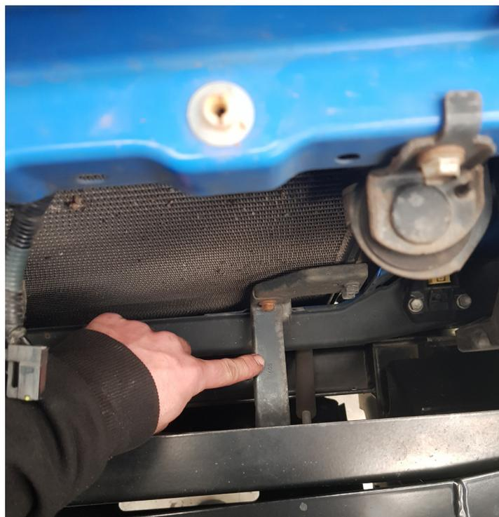
6. Remove the 10mm head bolt holding the radiator center support panel.
