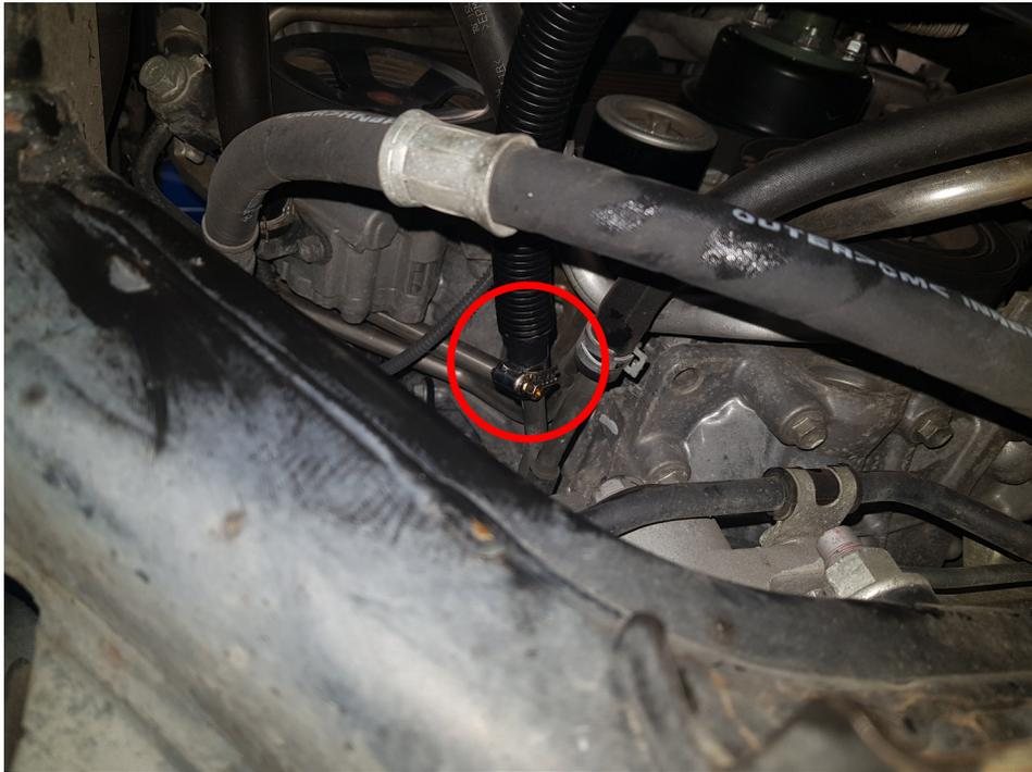
24. Secure the new hoses using the supplied (5) cable ties so that they are routed away from moving parts.
