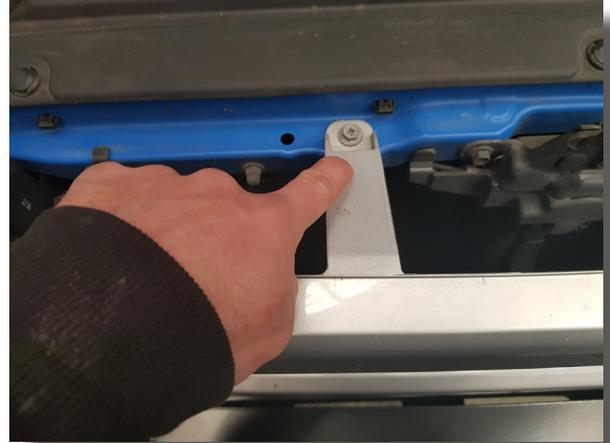
4. Remove the horn located on the passenger side of the top radiator support panel. Keep the bolt as you will use this in a later step.
