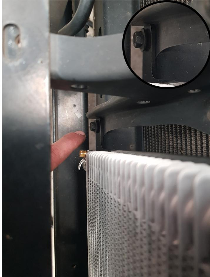
13. Install the plastic clip in the square hole of the angle bracket supplied with your cooler bracket. Bolt (use factory bolt removed earlier) the angle bracket and cooler bracket together to the vehicle via the bottom right hand bolt hole in the cooler bracket. Clip in air conditioning line. See photo below.
