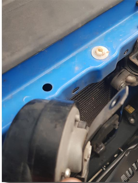
15. Bolt the supplied cooler bracket's top bolt hole and the horn (flipped to face the reverse direction) to the original horn mounting hole.
