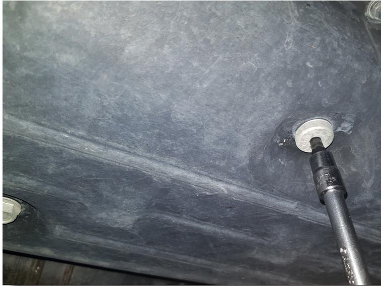
29. Using a small hose through the fill plug hole, pump oil into the transmission until it begins to come out of the check hole.
