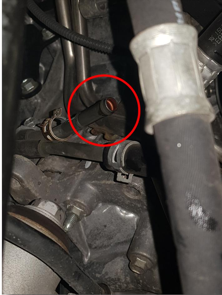
Cut the supplied cooler hoses to length, attach them to the factory steel pipes (it does not matter which hose is attached to which pipe as the cooler is unidirectional) and clamp with the (2) supplied hose clamps.
