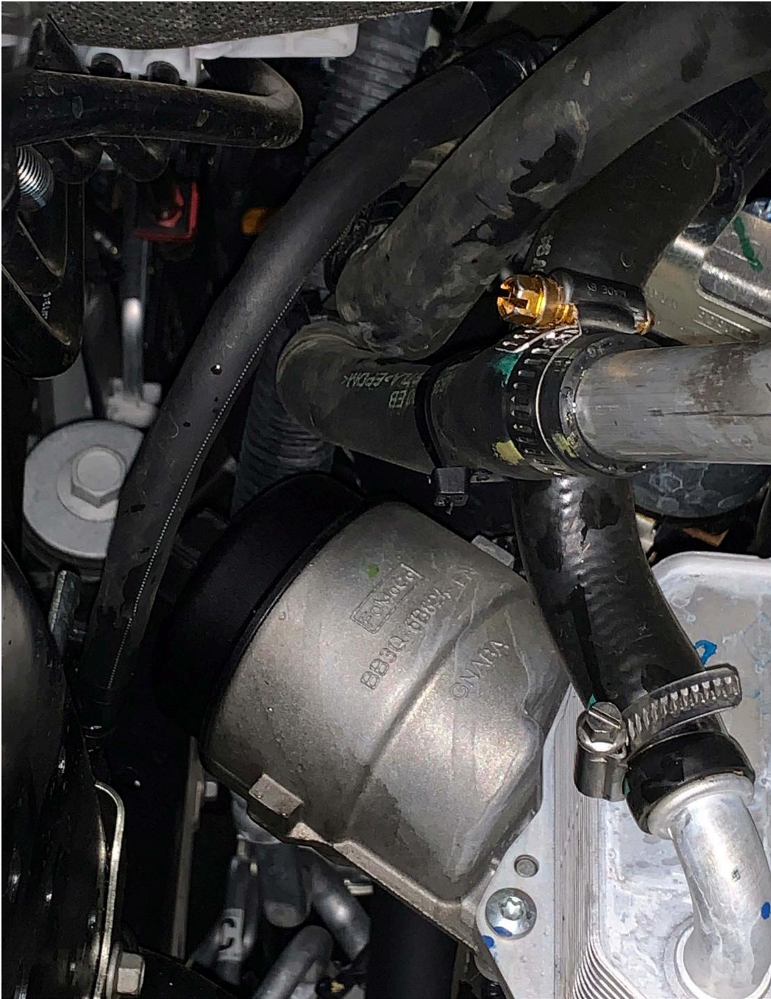
33. Recheck transmission coolers, fittings, hoses, unions, mountings and clamps for any loose fittings. Tighten if necessary.
