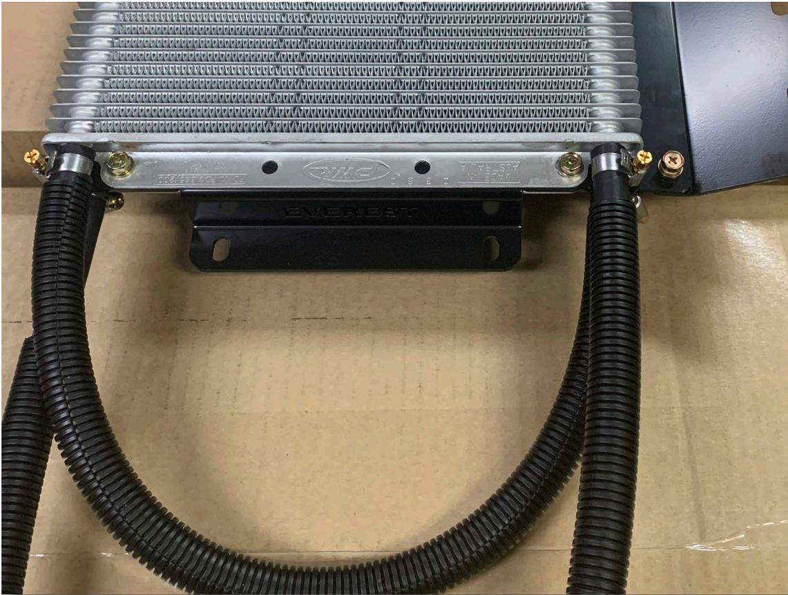
15. Lower the cooler assembly into the vehicle and place top of bracket behind radiator support panel, lined up with existing hole. Using 1 x M6x20 SEMS bolt, secure bracket to radiator support panel.
