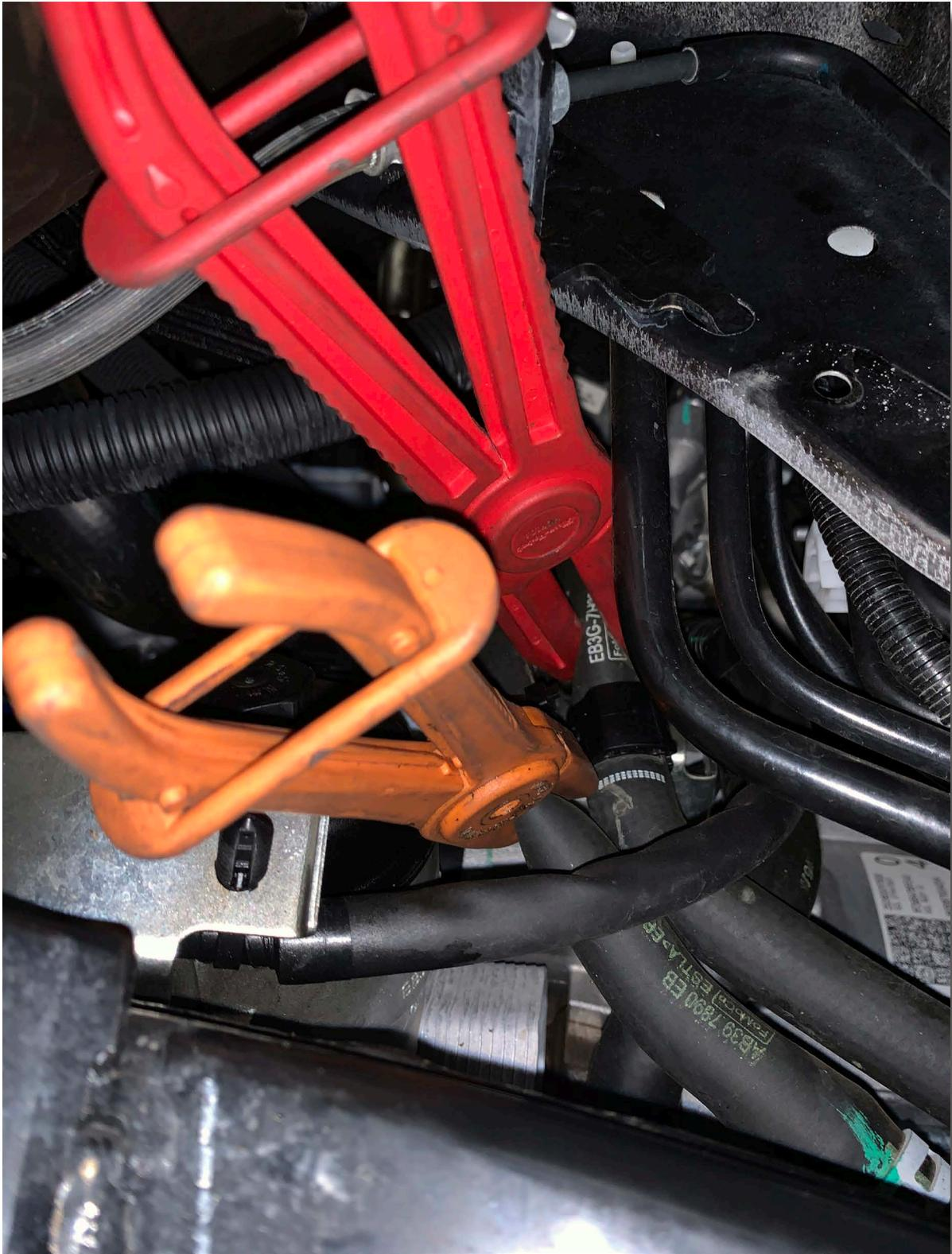
21. Remove coolant hose clamps and then remove the hoses from the heat exchanger. Make sure you have a drain tin or bucket under the hoses to catch the small amount of radiator fluid that will drop out.
