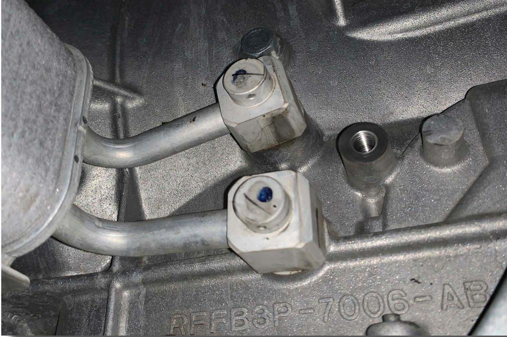
23. Unbolt heat exchanger by removing the three bolts holding it to the transmission. Two bolts are above the heat exchanger and one bolt below. All three bolts are either T40 Torx on newer models or 10mm hex head on older models. Do not discard the bolts.
