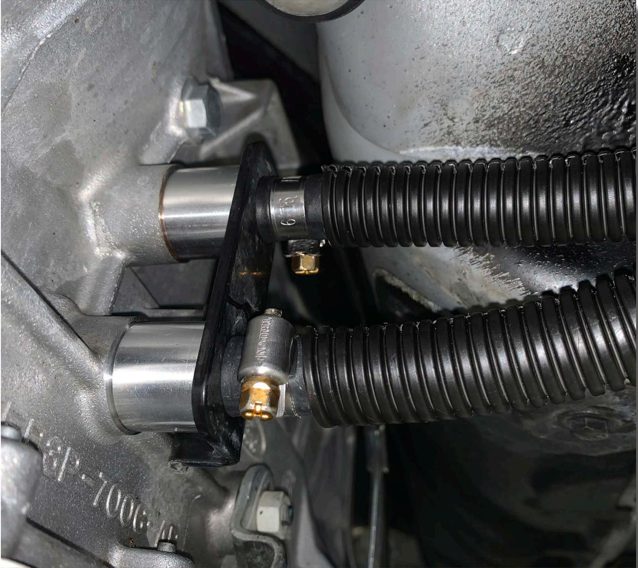
32. Check clearance of hoses to front prop shaft. Cable tie the coolant hoses to prevent rubbing.
