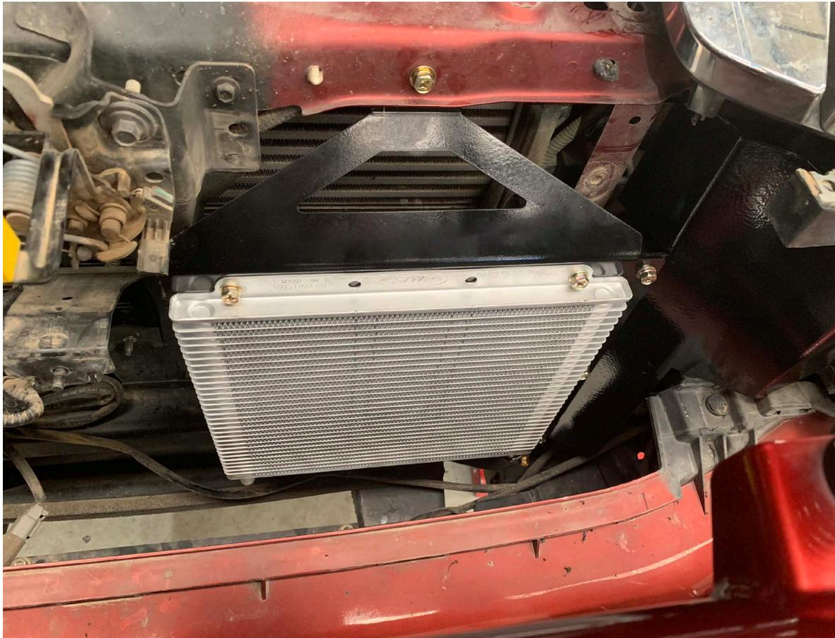
17. Re-Install the two (2) original drivers side shroud fixings. Using the supplied Shroud Mounting Bracket, fit onto the stud for the horn bracket then re-fit horn bracket and finger tighten with original nut. With supplied M6x20 SEMS bolt, fit through existing hole in shroud into the thread in the Shroud Mounting Bracket. Tighten both nut and bolt.
