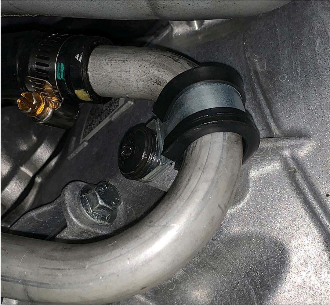
29. Check the routing of the cooler lines prior to cutting to ensure they will not impact on any part of the vehicle or could become jammed or pinched. Cable tie them so they keep sufficient clearance around the Engine Oil Filter for ease of engine maintenance.
