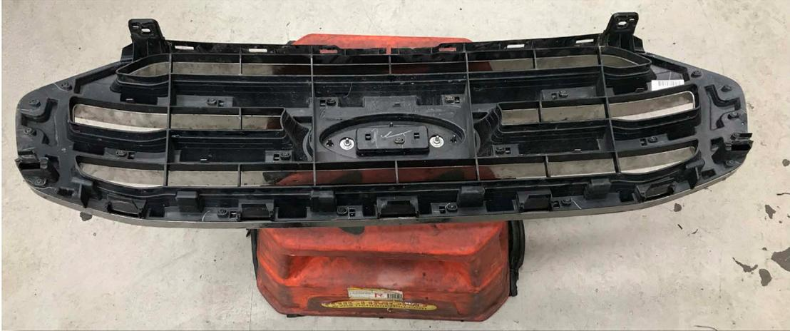
4. Remove the shroud from the bonnet release catch by removing the bolt on the drivers side and releasing the clip on the passenger side. Do not discard.
