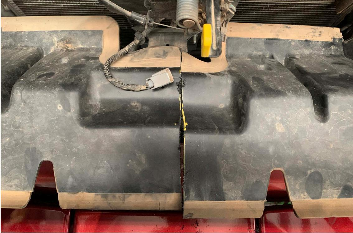
11. Drill an 8mm hole beside the original hole for the wiring clip. We will use the original hole for securing the shroud. The new hole is for the wiring clip.
