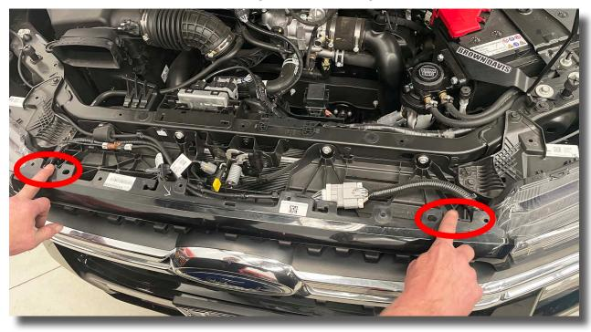
1.6. Disconnect the brown plug on the drivers side of the vehicle, and the water pipe in the center. Be sure to position the pipe ends so as to minimise loss of water.
