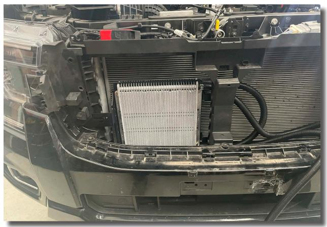
1.14. Using the M6 X 25 SEMS bolts supplied, mount the passenger side cooler bracket as shown below:
