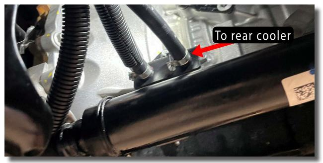
1.29. Secure using cable ties provided. Remove all clamps and replace the plastic panel that was removed from the wheel arch and refit bash plate.
