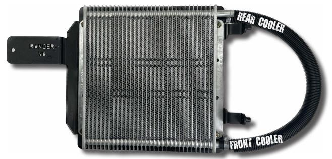
Coolers are omni-directional, so the direction of flow is not important. However for maximum efficiency and effectiveness we recommend the hot oil enters the rear cooler first.
