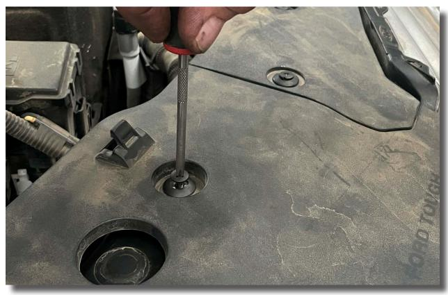
1.4. Using a T30 Torx bit, remove the screw holding the air inlet snorkel to allow you to easily remove and reinstall the radiator cover.
