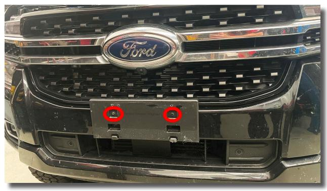
1.8. Working along the base of the grill, pull forward to dislodge the clips holding it in place. Clips can be difficult to dislodge and may need to be released from behind the grill
