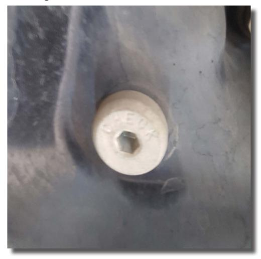
33. With the **engine running** remove the check valve bolt using a 5mm Allen key. DO NOT remove the 14mm bolt located at the rear of the transmission pan as this is the drain plug.
