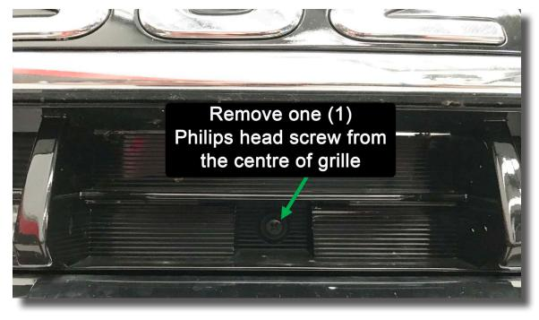
6. Remove the top half of the grill by firmly pulling forwards. Set aside.
