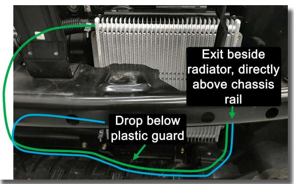
25. Route the hoses along the chassis rail until you reach the wheel arch. From wheel arch, route the cooler lines across to the side of the transmission and cable tie to the factory steel lines.
