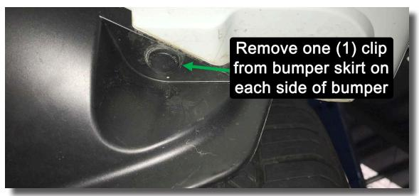
13. Find the two points where the front bumper skirt joins together, just in front of where the front tie down points are located. Slide the skirt apart and remove the final two hidden clips (one on each side).
