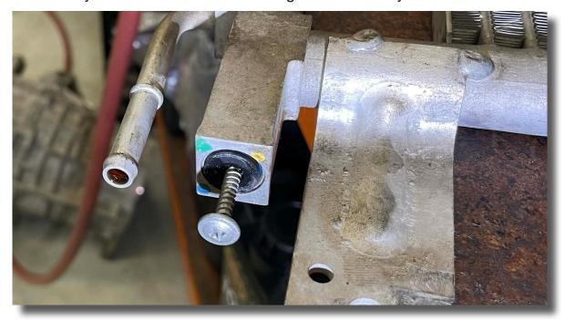
3.21. With the cap removed, extract the thermostat and spring if they aren't already out of the housing. The bypass valve does not require either of these parts to be reinstalled.
