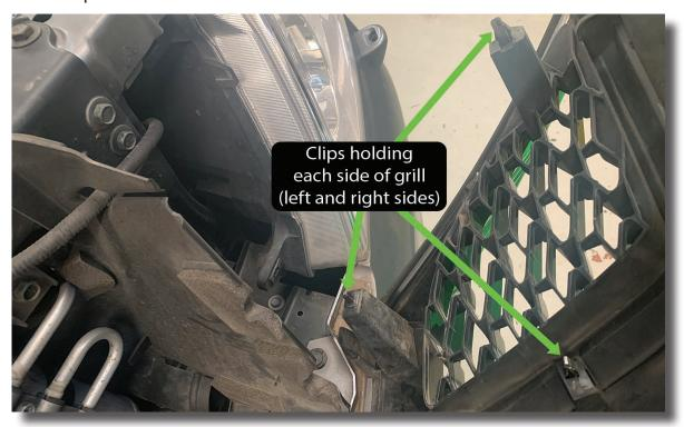
3.6. Remove the grill by gently lifting up on the 6x clips at the bottom of the grill.
