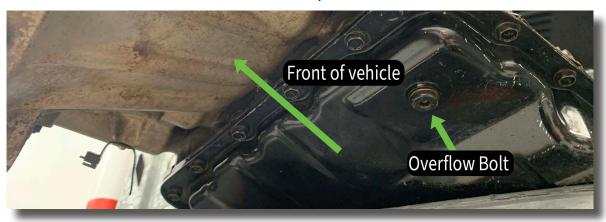
3.37. Once the engine has been running for at least 1 minute, move a drain tin into place under the overflow outlet and then remove the 5mm hex bolt. If the transmission fluid starts to flow out of the overflow tube in a light but steady stream (as indicated in the two following images), then there is sufficient fluid inside the transmission for the test drive. Wait until it slows to a dribble and reinstall the overflow bolt. You can now skip to step 3.42.
