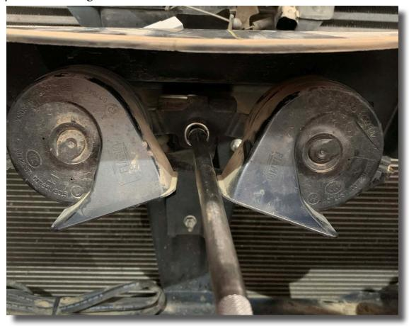
6. Mark a line from front to back as shown below. The line should be on the passenger side of the hole that was used to secure the bonnet release wiring.
