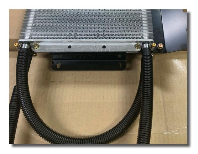
15. Lower the cooler assembly into the vehicle and place top of bracket behind radiator support panel, lined up with existing hole. Using 1 x M6x20 SEMS bolt, secure bracket to radiator support panel.
