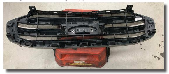
4. Remove the shroud from the bonnet release catch by removing the bolt on the drivers side and releasing the clip on the passenger side. Do not discard.
