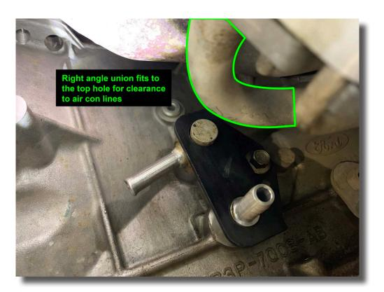
\*Note: If installing with a transmission temperature gauge, the union to use for for the temperature sensor (Hot Line) is the lower union.
