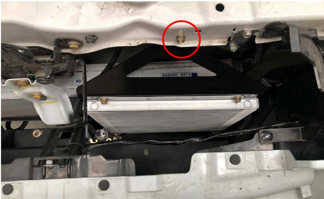
21. Refit the (1) 10mm head bolt that was earlier removed from the center brace on the bottom of the radiator support through the lower left cooler mount and back into its OEM hole located on the passenger side of the center brace of the lower radiator support.
