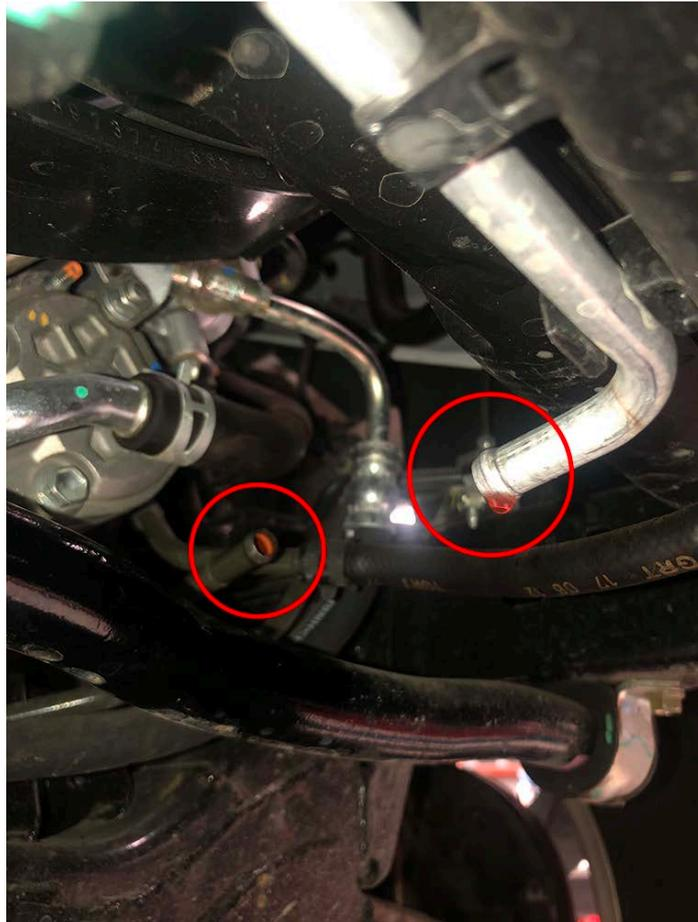
16. Remove the union fitting rubber socks from the supplied cooler.
