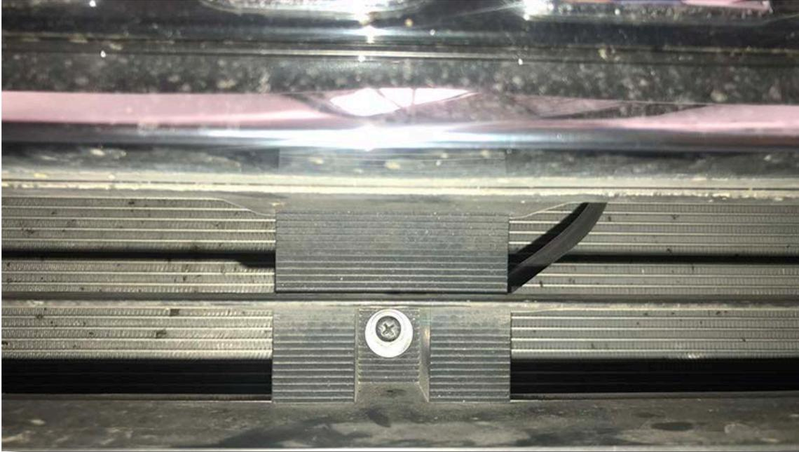
5. Lightly pull the front grill forward in order to access the two plastic tabs which hold it into the front bumper bar.
