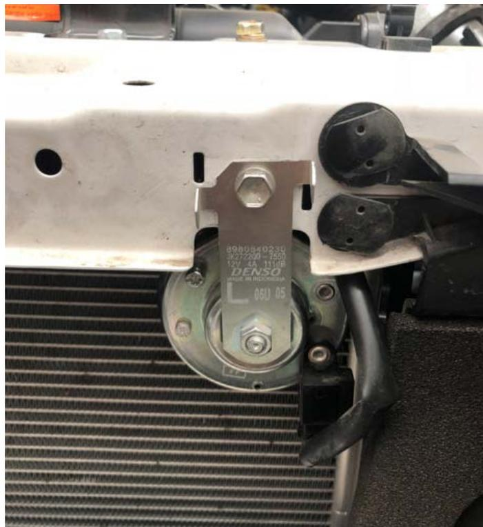
9. Remove the (1) 10mm bolt located in the center brace of the bottom radiator support on the passenger side of the vehicle.
