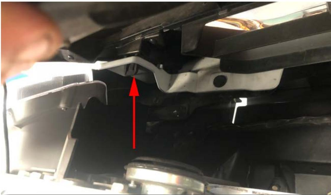
6. Gently undo the two plastic tabs by lightly lifting them up while holding forward pressure on the grill.
