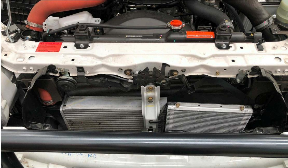
20. Using the (1) 10mm head bolt supplied, tighten the bolt into the top of the bracket through the top of the radiator support into the cooler bracket nutsert.
