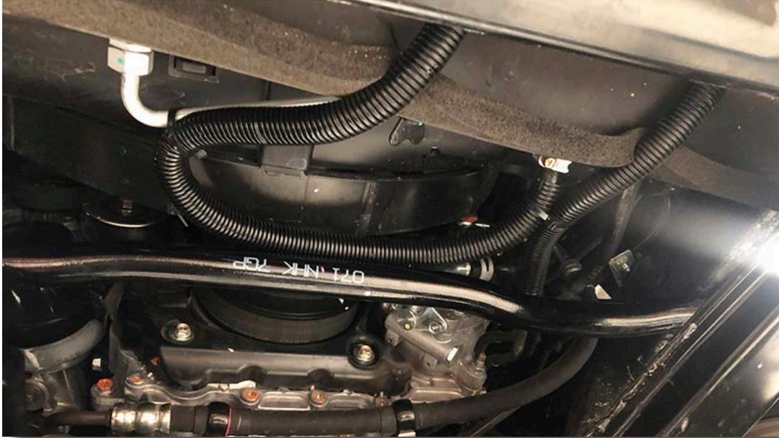
24. Roughly route each cooler line to either of the union fittings earlier exposed when the OEM rubber transmission hose was removed. The lines can be routed to either fitting - it does not matter which one. Cut off the excess rubber hose.
