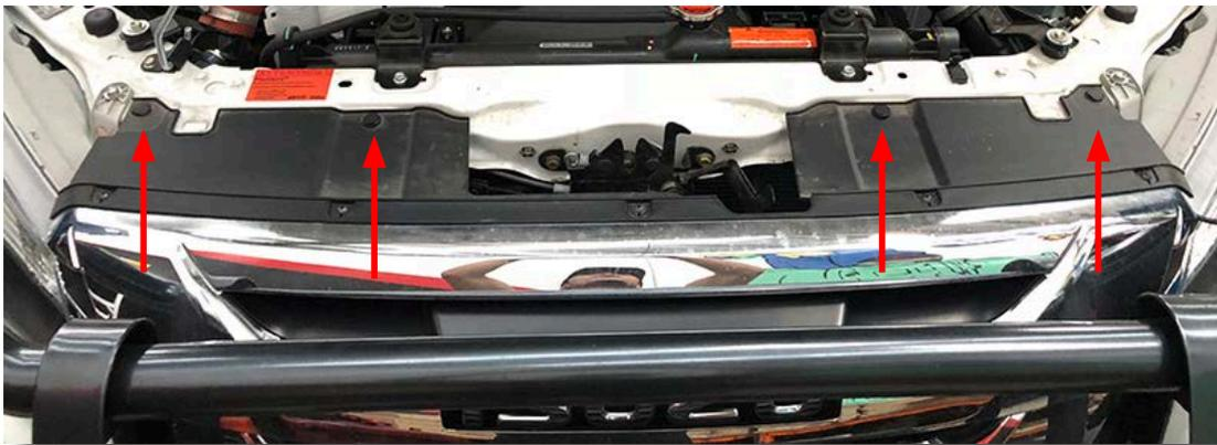
4. Remove the (1) Phillips head screw in the center of the grill located just under the Isuzu front badge.
