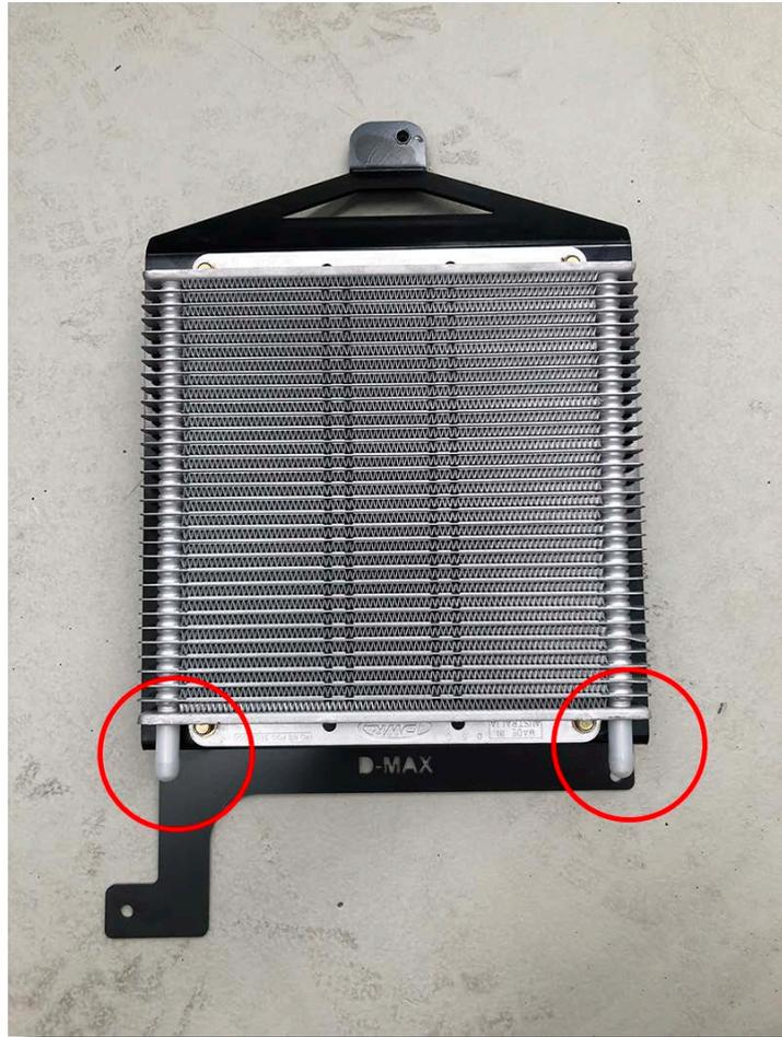
17. Cut the supplied rubber hose in half and fit each half to either of the union fittings on the supplied cooler. Do not use lubricant to fit these hoses.
