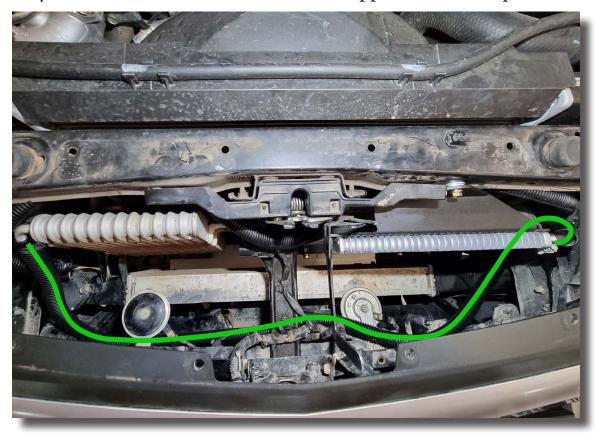
41. Connect the second half of the cooler hose to the bottom port of the cooler core and secure it with one of the supplied hose clamps.
