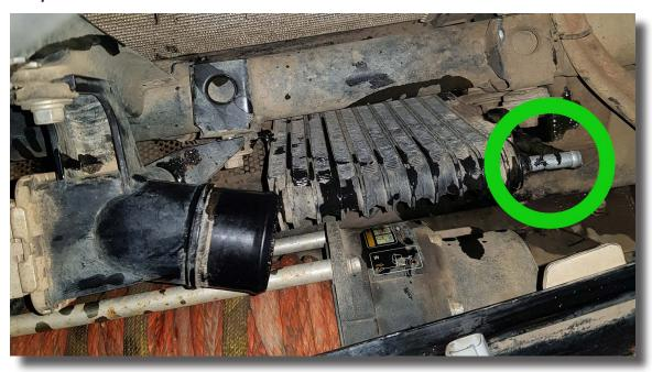
6. Loosen the bolts indicated in the photo below, but do not remove them. One bolt attaches the intercooler to the lower radiator support panel. The second bolt attaches the OEM oil cooler to the lower radiator support panel.
