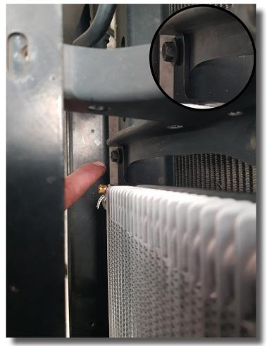
13. Install the plastic clip in the square hole of the angle bracket supplied with your cooler bracket. Bolt (use factory bolt removed earlier) the angle bracket and cooler bracket together to the vehicle via the bottom right hand bolt hole in the cooler bracket. Clip in air conditioning line. See photo below.
