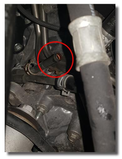
Cut the supplied cooler hoses to length, attach them to the factory steel pipes (it does not matter which hose is attached to which pipe as the cooler is unidirectional) and clamp with the (2) supplied hose clamps.
