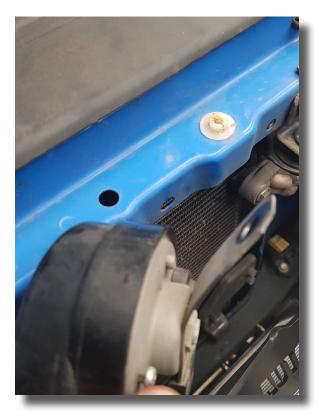
15. Bolt the supplied cooler bracket's top bolt hole and the horn (flipped to face the reverse direction) to the original horn mounting hole.
