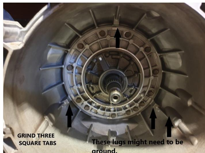
*In the course of fitting the Torque Converter it is vital that the person fitting such a unit determines that there is sufficient end clearance between the crankshaft and front pump to allow the converter to spin freely.*
