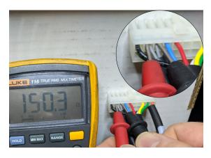
3. If the resistance is not 18,000 ohms (18k)then please contact your place of purchase or you may gently pull the two grey wires from the sheathe to reveal the resister. Remove the factory resistor and replace with 18,000 ohm (18k) resister.
