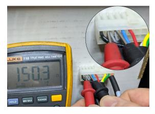
3. If the resistance is not 820 ohms then please contact your place of purchase or you may gently pull the two grey wires from the sheathe to reveal the resister. Remove the factory resistor and replace with 820 ohm resister.
