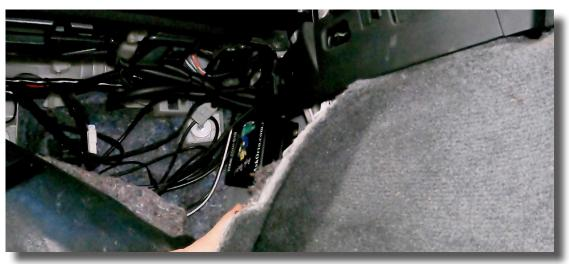
3.1.5 If the GEN2 Module has been screwed to the transmission tunnel, use a screwdriver or drill to remove the GEN2 Module and disconnect from loom.
