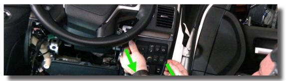
3.1.15 Now returning to passenger side, use a coat hanger or push wire, tape the CANBUS terminal ends to the coat hanger. Approx 50cm from the switch connector, loop the leg and tape to the coat hanger also.
